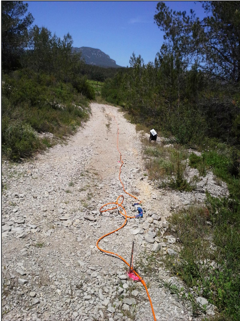
Picture of the CRITEX ERT equipment in use on Cretaceous limestones (Le Triadou, France).
