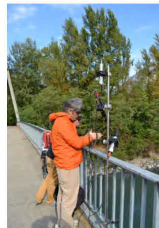
Fig. d: Measurement of optical properties of water using radiometers.
