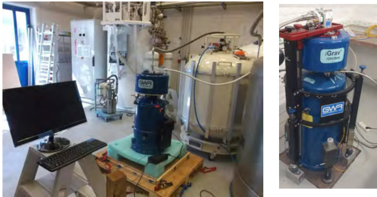
iGrav superconducting gravimeter (during a liquid helium filling on the left and installed on a pillar at the Strasbourg Gravimetric Observatory).
