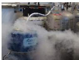
Figure 5 : Liquid helium refilling at cryogenic department
