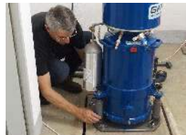
Figure 6 : Set-up of thermal levelers to compensate tilt changes
