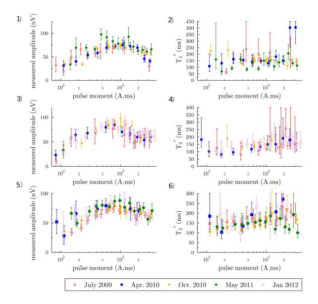
Figure 4: Temporal variability of MRS signals. Signal amplitude e (left) and apparent transverse relaxation time  $T_2^*$  (right) of the MRS signals as a function of the energizing pulse, for sounding performed at Menu (graphs 1, 2), H2 (graphs 3, 4) and H3 (graphs 5, 6) sites. Only pulses with a S/N greater than 1.5 have been used for the apparent relaxation time graphs.
