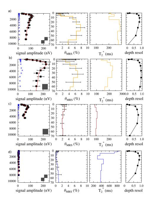
Figure 8: Example of MRS signal and inversion for selected sites: a) Chou (ruiniform dolomite, eight square loop), b) Cana (ruiniform dolomite, square loop), c) SambH (siliceous limestone, square loop), d) CombR (marly limestone, eight square loop). MRS results plots (left): signal amplitude e (squares), ambient noise measurements (crosses), MRS inversion (line).
