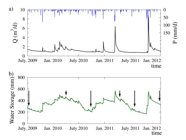
Figure 5: Water storage change on the Durzon catchment: a) Daily rainfall and measured Durzon spring discharge, b) Simulated water storage change on the Durzon catchment. Arrows stand for MRS field campaigns. The water storage at July 1st 2009 is arbitrarily set to zero.
