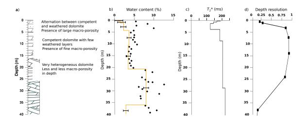
Figure 7: Comparison of MRS results and core samples from a drillhole performed at the center of H3 site: a) simplified log resulting from a synthesis of visual observations performed on 3 different boreholes, b) core sample water content (markers), and MRS (% - line), c)  $T_2^*(z)$  (ms), d) depth resolution of the MRS model.
