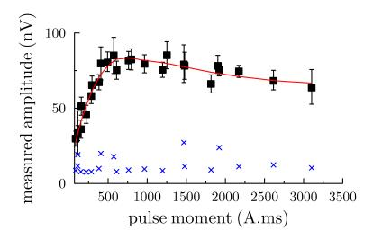
Figure 6: MRS signal and inversion results on H3 site. Square: signal amplitude e. Cross: ambient noise measurements. Line: MRS inversion.
