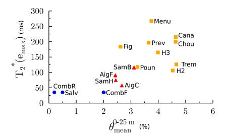
Figure 9:  $T_2^*(e_{max})$  as a function of  $\theta_{mean}^{0-25m}$  for soundings performed in ruiniform dolomite (squares), siliceous limestones (triangles), and marly limestone (circles). For marly limestones,  $T_2^*(e_{max})$  is set to 35 ms referring to the instrumental dead time of the device, and  $\theta_{mean}^{0-25m}$  is set equal to the maximum water content.
